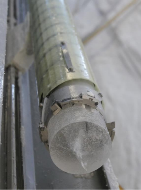
Ice core from the brittle zone, with orientation mark on core, and side force spring mounted on outer core barrel, July, 2017.
