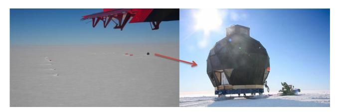
Left: Fly over photo of the stored NEEM camp May 2013. The line to the left is sledges with equipment stored and the black building to the right is the main dome on skis. In the two red tents the tracked vehicles are stored. Right: Photo from 2011 of the 4 storey, 45 ton main dome on skis being pulled by the NEEM Pistenbully.
