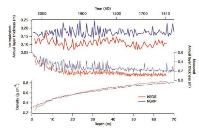
Reconstruction of the annual layer thickness from the 67 m shallow ice core from NEGIS. The accumulation rate is 0.11 m/yr and a significant increase of accumulation in the more recent warmer years is not observed. The results are compared with records from NGRIP. (P.Vallelonga et al, Preliminary glaciochemical and geophysical study of the Northeast Greenland Ice Stream (NEGIS), submitted to the Cryosphere)
