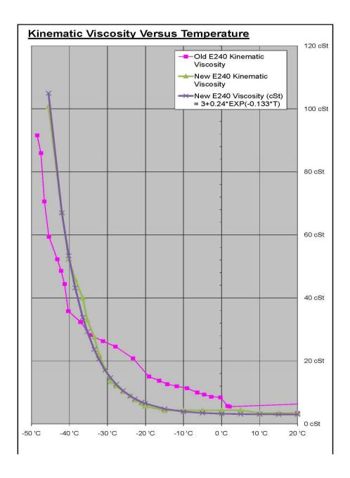
In February 2008, the supplier of Estisol 240 announced a change in specifications of the fluid due to a change in raw materials for the production (coconut oil has become too expensive) We therefore conducted a new set of measurements. As seen above, by cheer luck, this change has improved the fluid for our use. Purple: old Estisol 240; Green: New Estosol 240. Blue: simple model of kinematic viscosity vs. temperature.
