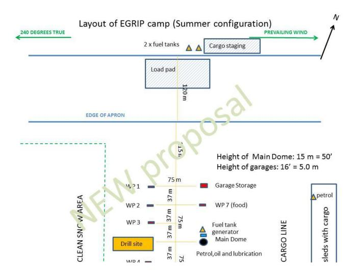
This new proposal was negotiated with the109th to meet with their desire to park the air craft into the wind. Bcause of the location of the fuel point on the starboard side of the plane, the fuel tanks have to be on the skiway side of the apron. The advanteage is that passengers leaving and entering the plane can walk straight to/from camp.
