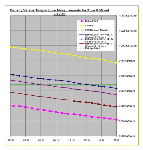
Above - density versus temperature of the drilling liquids in pure & in different mixes.
