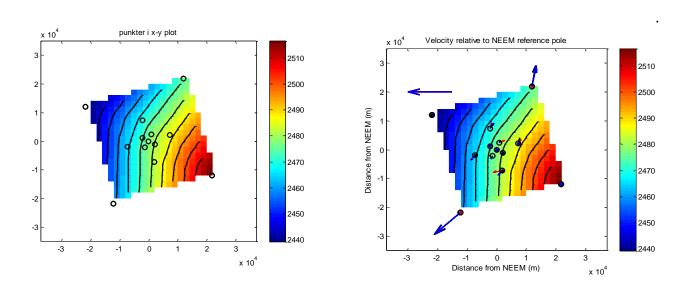
Fig. Left: Map of existing strain net at NEEM. The circles indicate poles. It is of high priority to remeasure the filled poles. The purple circle indicates the reference pole at NEEM. Right: Arrows indicate horizontal surface velocities relative to the NEEM reference pole over the period 2007-2008 (red), 2008-2009 (black), 2009-2010 (blue).
