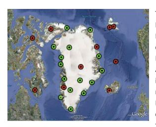
1 The map shows the location of existing real-time broadband seismic stations (red) joining GLISN with open data sharing and sites (green) where equipment, telemetry, and infrastructure is being installed and upgraded in concert with GLISN partners.
