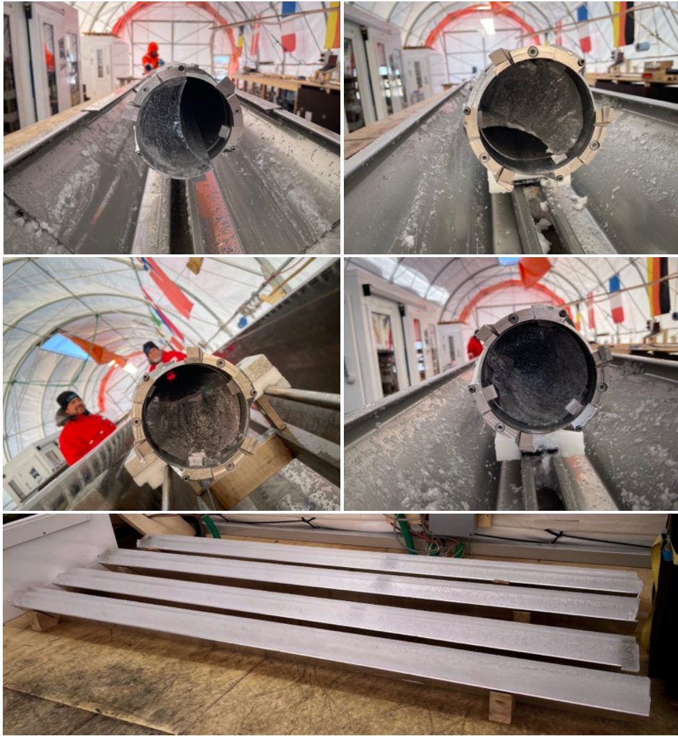
The half-moon shaped core slowly grew to a full core (in lower picture from back to front). Photos by B. Seth
