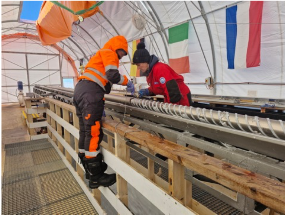
Iben and Barbara decoupling the core barrel from the super banger after a filter run. Photo by H. Traeger
