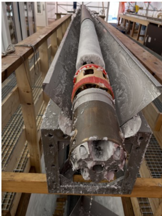
The result of one of our filter runs: the chips chamber full of coarse chips. Photo by B. Seth
