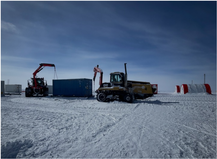
The two Challengers lifting the containers on sledges. Photo by B. Seth
