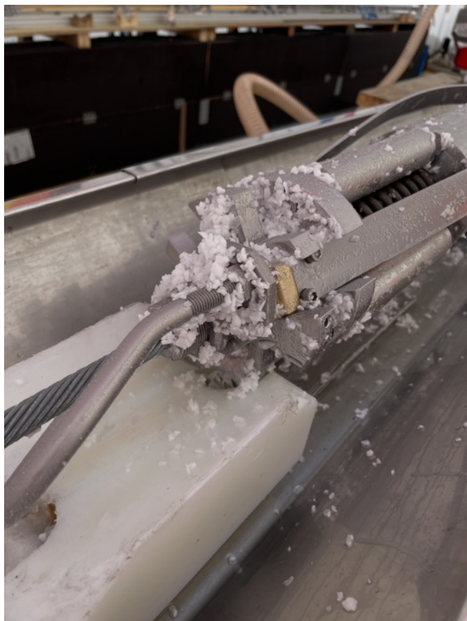
Coarse chips on top of the antitorque. Photo by B. Seth
