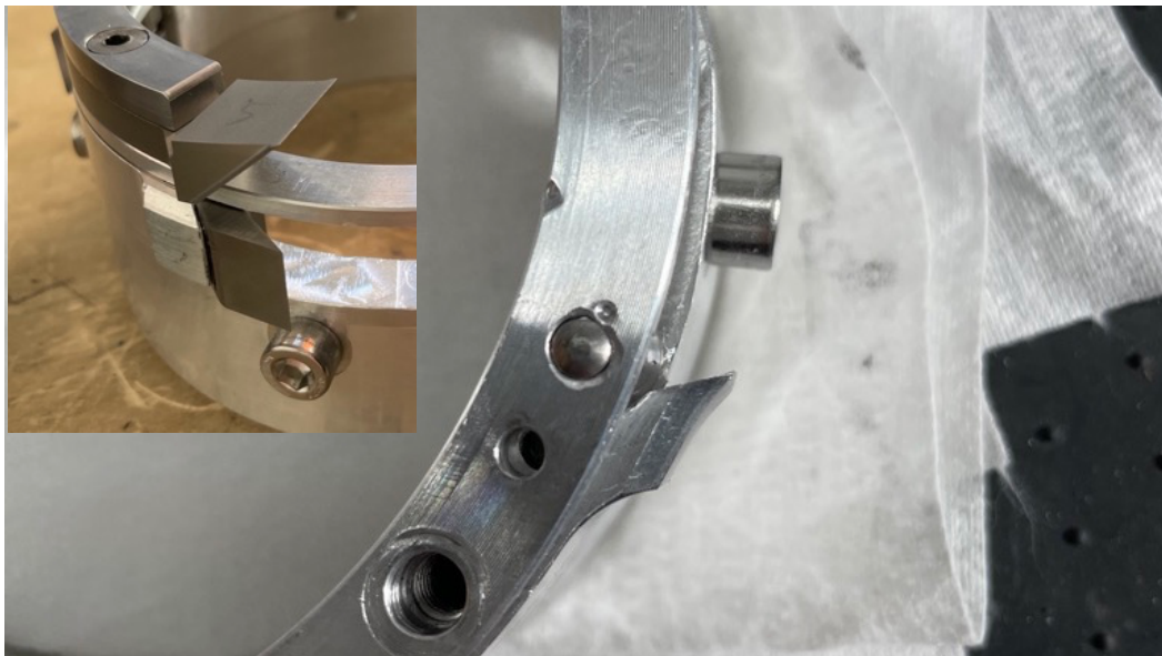
The large picture shows the bended end-stop for the catchers (already dismounted); the small picture shows the drill head with mounted cutters and lateral catchers before use. Photos by B. Seth
