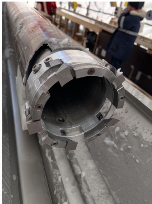
The modified ‘Coretters’ mounted on the 2.5 m core barrel. Photo by B. Seth
