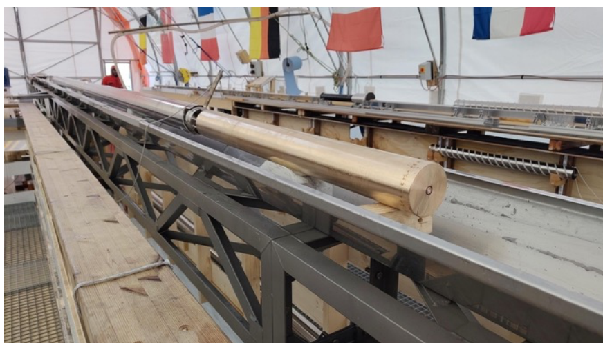
The new, 70 kg dead weight mounted underneath the valve will hang inside the core barrel. Photo by K. Ederer
