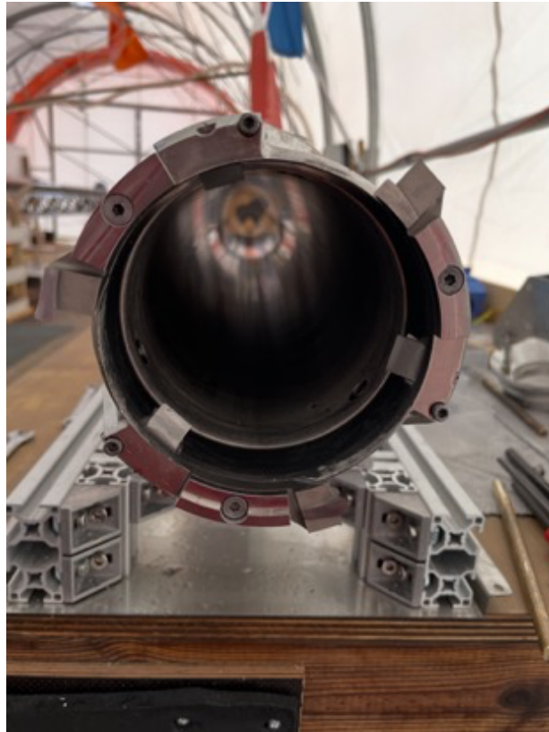
The normal ice drill head with stepped cutters resting on the logging table. Photo by B. Seth.
