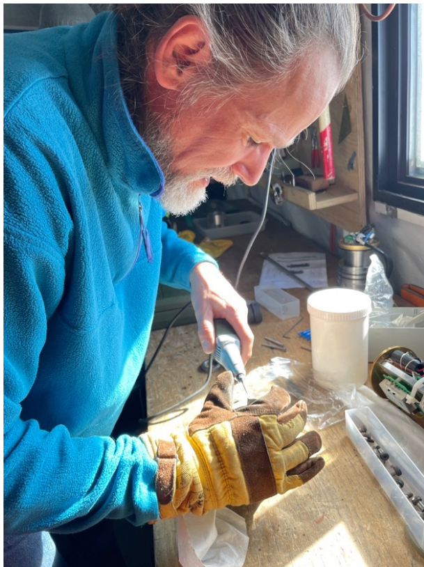
Gunther sharpening the outer edges of the cutters on the drill head. Pictures: B. Seth Photo by B. Seth.
