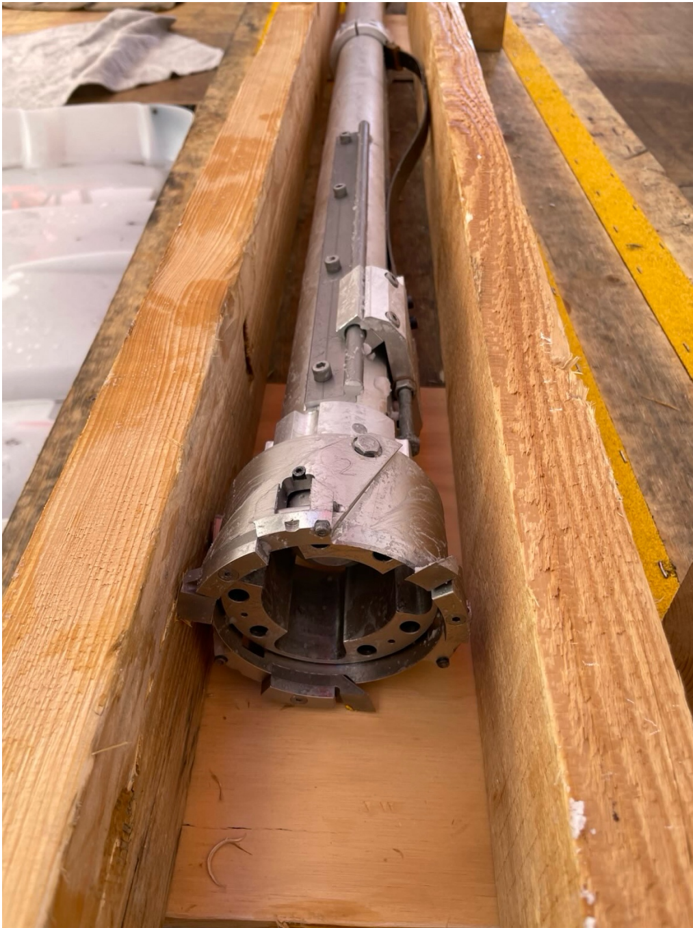
Testing the deviation tool with the wooden construction that should represent our hole. Here, it is obvious that the spring on the deviation tool was much too tense.. Photo by B. Seth.
