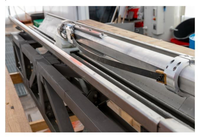
The deviation tool with the spring on the side and the drill head in the back as designed by the Copenhagen group. The spring is supposed to fit into the freshly broached groove down there in our bore hole at approximately 2327 m to 2352 m depth. Hence, the spring pushes the drill head to the opposite side of the bore hole to "ream"/mill into the wall and produce the wanted ledge.. Photo by G. Lawer.
