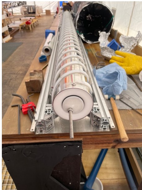
The white valve at bottom of drill opens when touching the ground (graft will be pushed in like a cork and fluid gets out, so the idea). Let's see if it work. Photo, B. Seth
