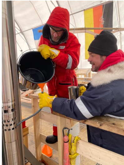
Highly sophisticated science 😊 to fill the lowermost part of the borehole with 165-Estisol, the high density drilling fluid. Photo B. Seth and K. Ederer
