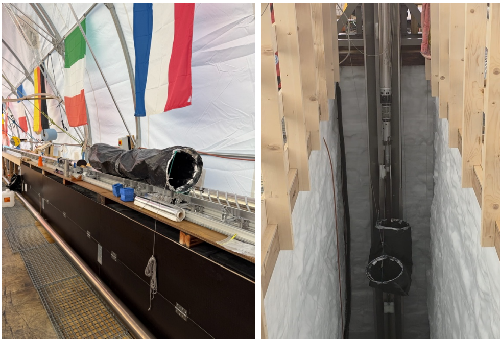
The shield protection of the drill core, "The sausage", lying on the logging bench, and in use when the drill core pops up at the surface. The full operation implies the synchronization of about three person maneuvering a set of four cords like professional puppeteers. Photo, C. Barbante, G. Bianchi Fasani
