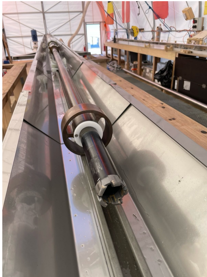
The Beyond EPICA rock drill head ready to be deployed in the abysses. Photo: B. Seth
