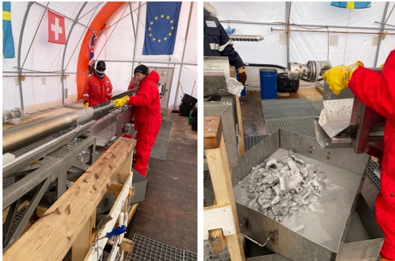
Filtrations of the drilling liquid in the drilling trench, Photo: B. Seth
