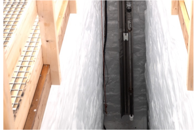
Rockdrill with a conical tool at the tip of the core barrel. Credit: F. Wilhelms ©PNRA/IPEV
