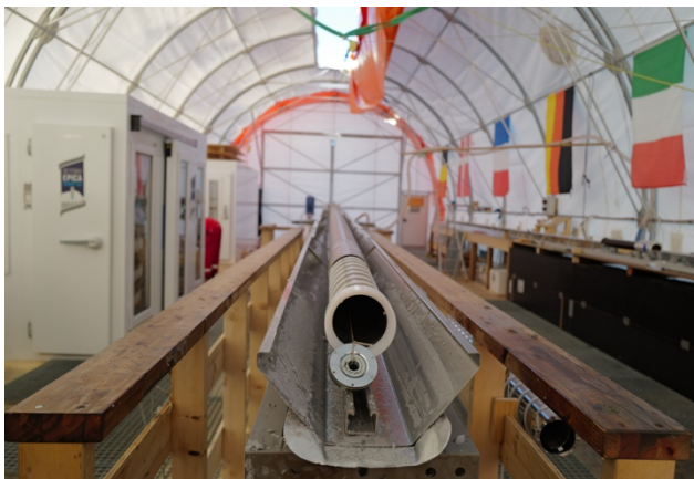
Wider conical tool with strong magnet attached to the ice core drill. Credit: F. Wilhelms ©PNRA/IPEV
