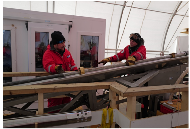
The assembled rock drill on the tower. FLTR: the outer core barrel, joint to the extension tubes, extension tube with brass centering ring, upper tube with super banger centering brass piece, super banger adaptor mount with milled pass-way and a part of the pump. Credit: F. Wilhelms ©PNRA/IPEV
