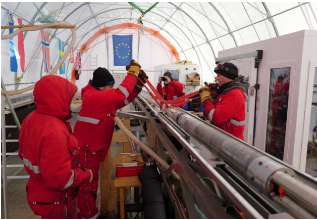
Mounting the rock drill string. Credit: F. Wilhelms ©PNRA/IPEV
