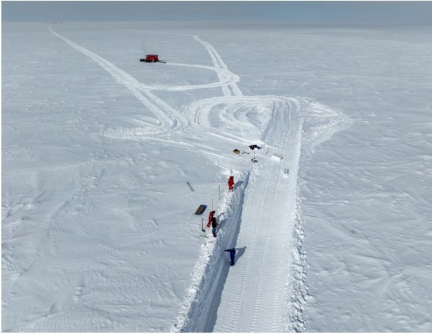
Overview of the 50 m trench for spatial variability studies as requested by the stable water isotope consortium. Credit: G. Lawer ©PNRA/IPEV
