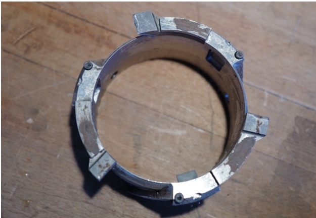
Worn cutter and debris frozen to the drill head during run #898 without penetration. Credit: F. Wilhelms ©PNRA/IPEV
