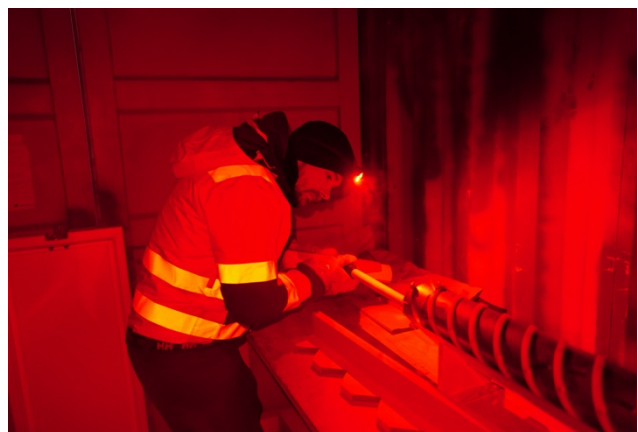
Pushing out the core in the red-light. Credit: F. Wilhelms ©PNRA/IPEV
