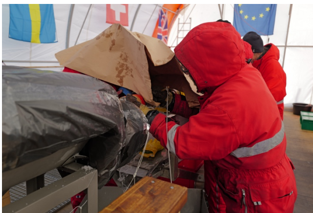
Unlatching the core barrel and putting a top plug. Shielded in the dark with a paper bag. Credit: F. Wilhelms ©PNRA/IPEV
