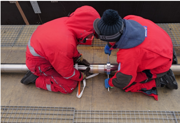
Lemmi and Barabara disassembling the 4m drill. Credit: F. Wilhelms ©PNRA/IPEV
