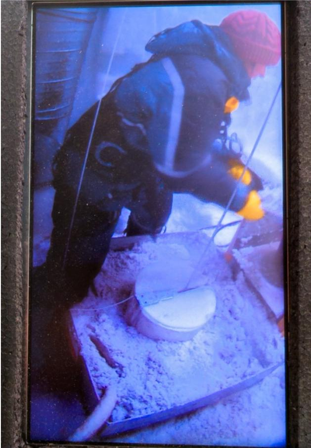
Lison as seen in the camera from the driller's operating desk while cleaning of the slush pan. Credit: G. Lawer ©PNRA/IPEV
