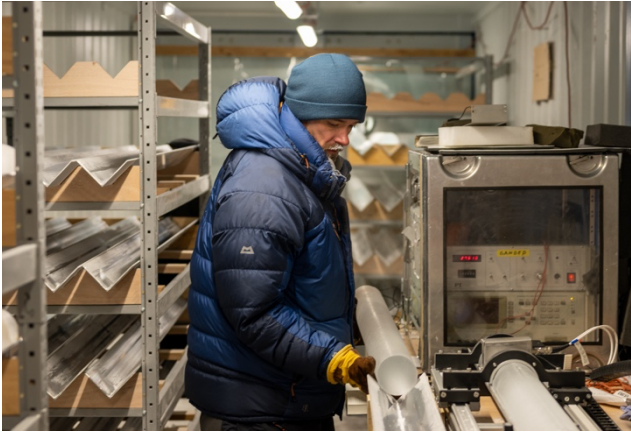
Impressions from the core processing marathon the two days before: Preparing the DEP (dielectric profiling) scan. Credit: G. Lawer ©PNRA/IPEV
