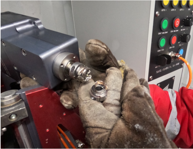
The broken coupling on the Swiss Saw. Spare pieces were available, and it was fixed in no time. Credit: J. Westhoff ©PNRA/IPEV
