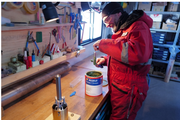
Lemmi, greasing the logger for good thermal contact, with the pressure housing in front. Credit: F. Wilhelms ©PNRA/IPEV
