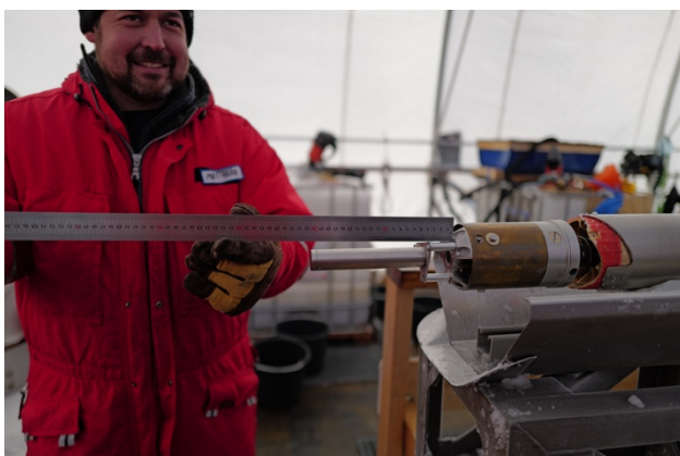
The mounted pressure housing attached to the super-banger. At the price of 20.5 cm less core. Credit: F. Wilhelms ©PNRA/IPEV
