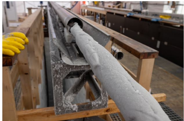
Upper end of slush recovered from the filter run. Credit: G. Lawer ©PNRA/IPEV
