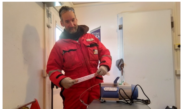
Lemmi, uses a medical rectal tube, to build an adaptor to connect the pump to the PICARRO. Credit: M. Bouchet ©PNRA/IPEV
