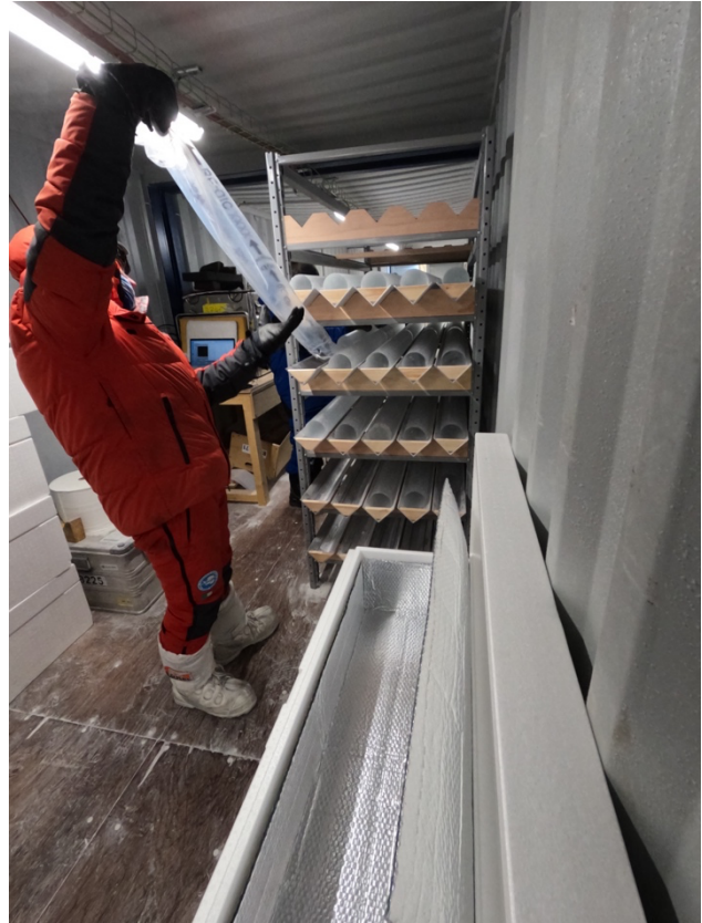
Federico (and Lisa behind the shelf) unpacking the ice cores in the core buffer. Here the cores will rest for 2 days, before processing. Credit: J. Westhoff ©PNRA/IPEV
