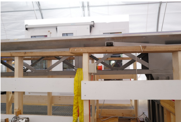
Martin mounted an additional emergency stop button, directly opposite of the tower control, where usually the second driller sojourns while operating the tower.
