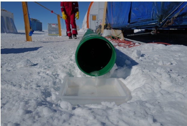
First version of a heat box from casing tubes for complete de-icing of the drill's shaft. F. Wilhelms ©PNRA/IPEV
