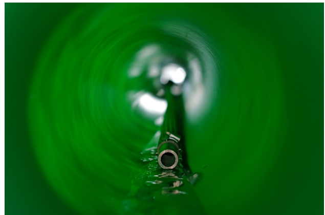
The drill-shaft in the casing tube. Credit: F. Wilhelms ©PNRA/IPEV
