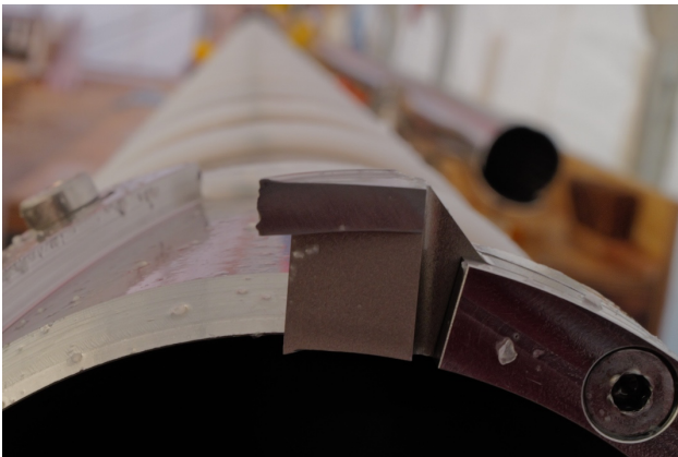
Worn outer step cutter after roughly 200 m of drilling. Credit: F. Wilhelms ©PNRA/IPEV
