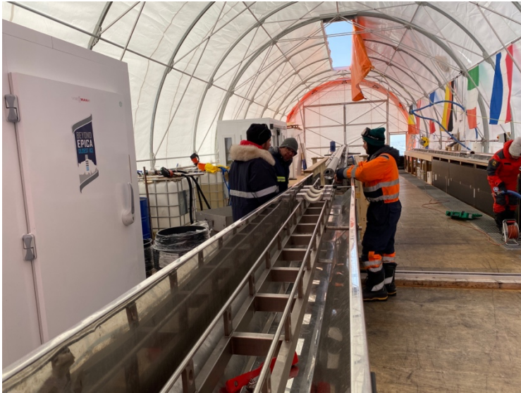
Figure 1: Matthias, Philippe and James aligning the extraction table: photo O. Alemany
