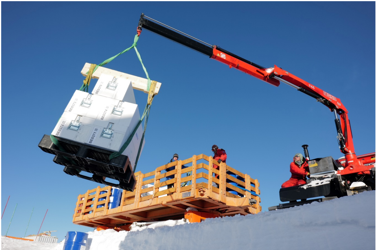
Lifting ice core boxes from the core buffer onto a trailer to transport them to Concordia for long-term storage. (Photo: Mulvaney, Leica SL2-S, 36mm, 1/200, f8, ISO100)
