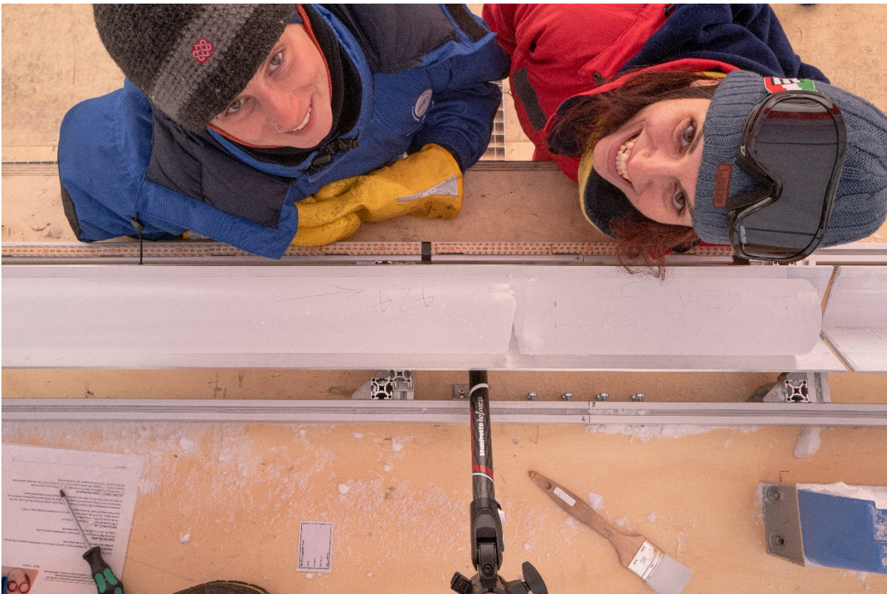
Giuditta (right) and Romilly (left) with bag number 424 on the cutting bench. The break in the ice is the join between two runs of the drill. (Photo: Mulvaney. Leica Q2, 28mm, 1/250, f11, ISO1250)
