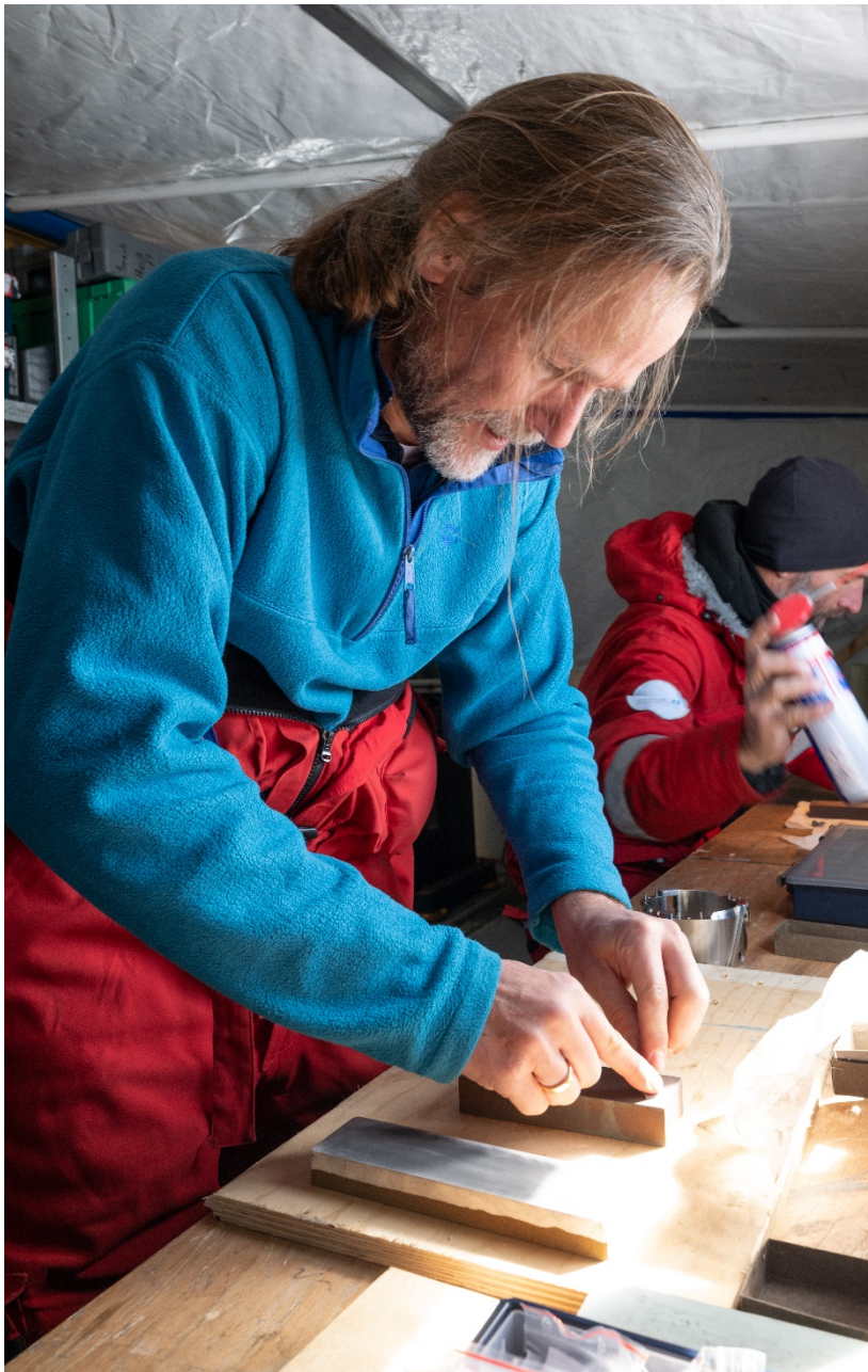
Gunther carefully sharpens the cutters for the drill head using a series of coarse to fine carborundum stones. (Photo: Mulvaney, Leica SL2, 25mm, 1/50, F8, ISO500)
