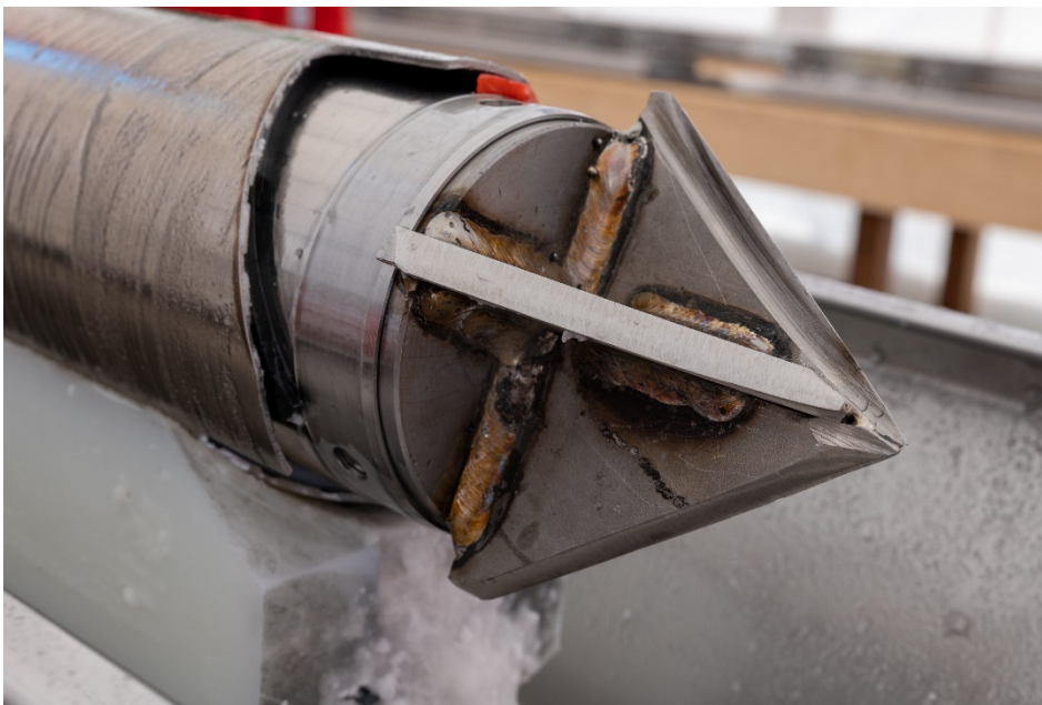
Arnold – the hardened steel cone cutter designed to isolate any debris in the borehole into a cone-shaped indentation on the top of the next ice core drilled. (Photo: Mulvaney, Leica SL2-S, 50mm, 1/100, f11, ISO400)
