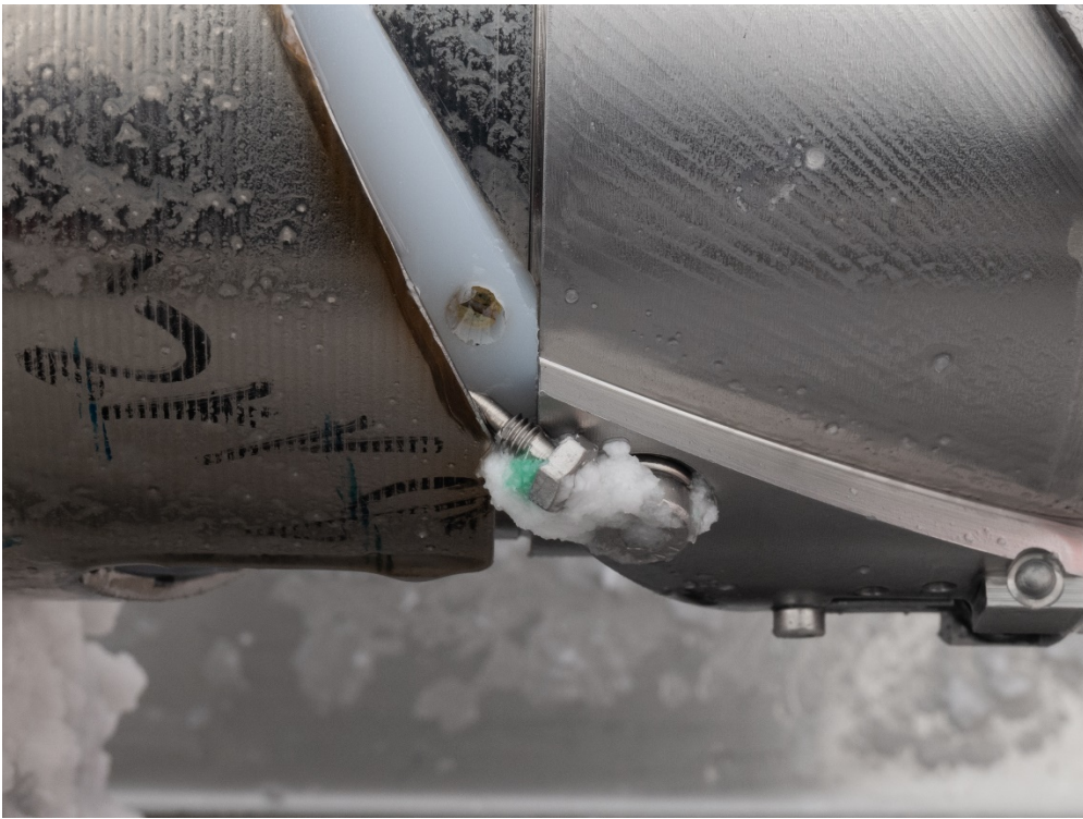
Close-up of the lost screw from the locking pin, jammed between the inner and outer barrel. (Photo: Mulvaney, Leica SL2, 35mm, 1/25, f11, ISO400)
