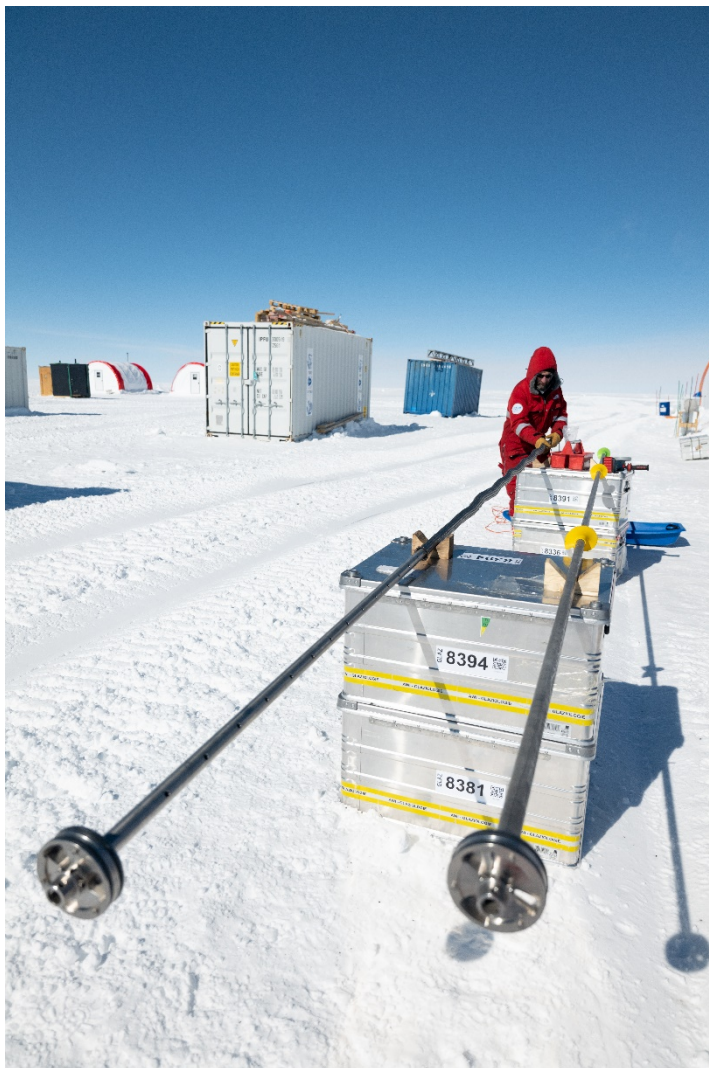
Lemmi prepares the hollow shafts for the long AWI drill which has a 4 m long core barrel. (Photo: Mulvaney, Leica SL2, 24mm, 1/16000, f4.211, ISO800)
