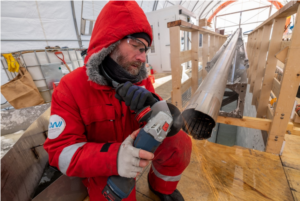
Lemmie cuts away part of the lower outer barrel to make triangular slots to better capture the chips produced by the drill head, directing them more efficiently to be captured by the spirals on the inner core barrel. (Photo: Leonhardt, Leica SL2, 16mm, 1/160, f8, ISO400)
