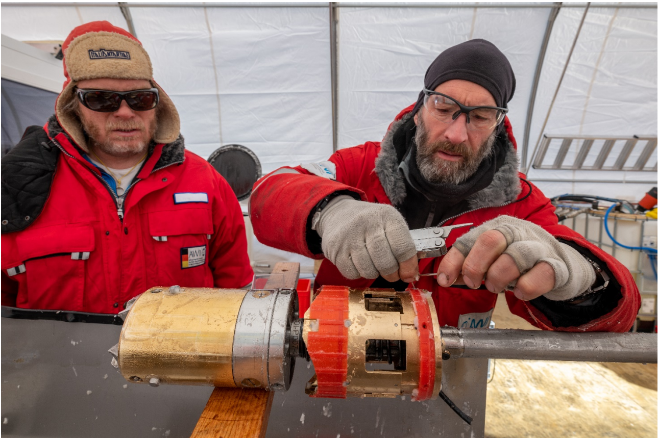
Lemmie adjusts the AWI fluid pump while Frank looks on; to the left of the fluid pump is the connector that holds the core barrel, while to the right of the pump is the lowest part of the 'hollow shaft'. (Photo: Mulvaney, Leica SL2, 16mm, 1/60, f8, ISO100)
