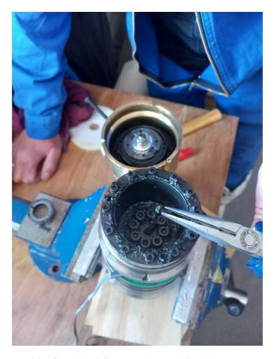
The cup of the gear with lot of metal shards from screws, bearing-balls and bearing cages mixed with the oil.
