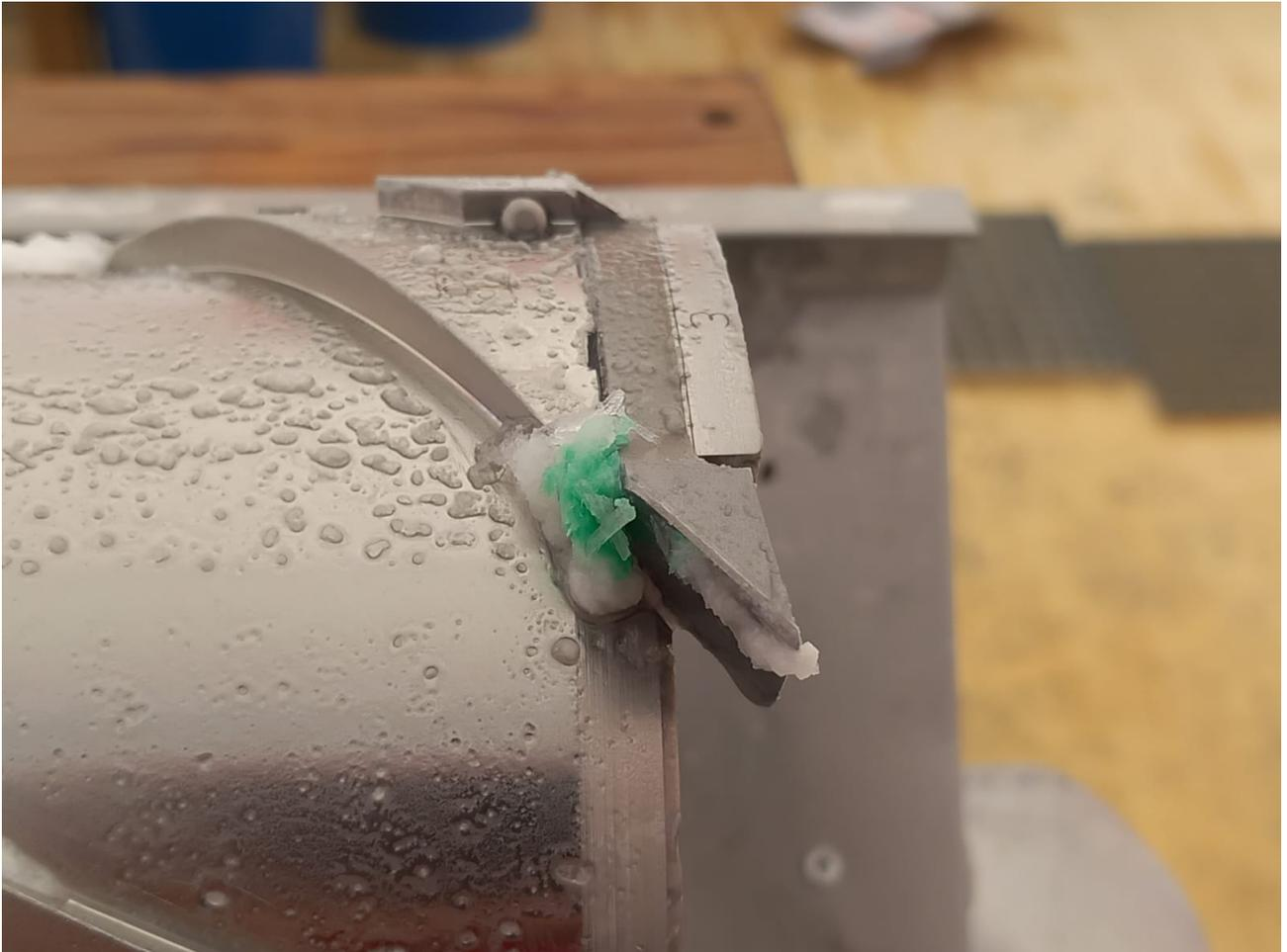
A detail of the drill head with some plastic pieces coming from the casing tubes.
