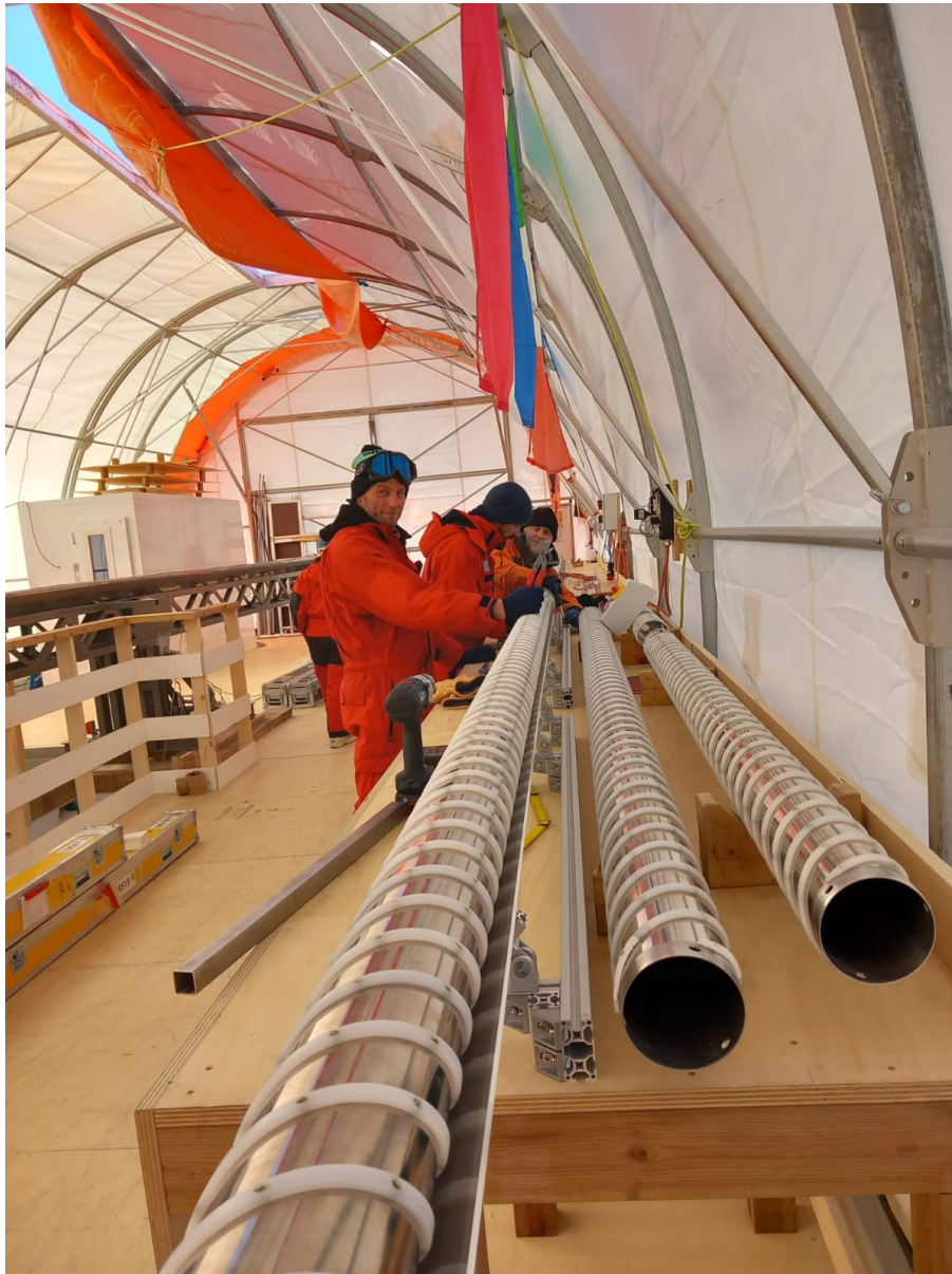
Alignment of the core extraction table and electrical wiring of the FED (fluid extraction device)
