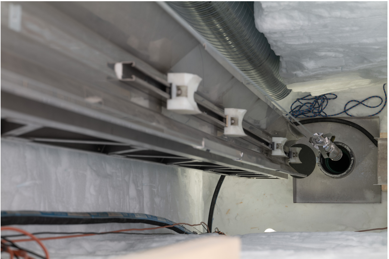
BEOIC drill being lowered into the bore hole. Photo: C. Barbante (Leica SL2, 90 mm, f 8, 1/25 s, ISO-200).
