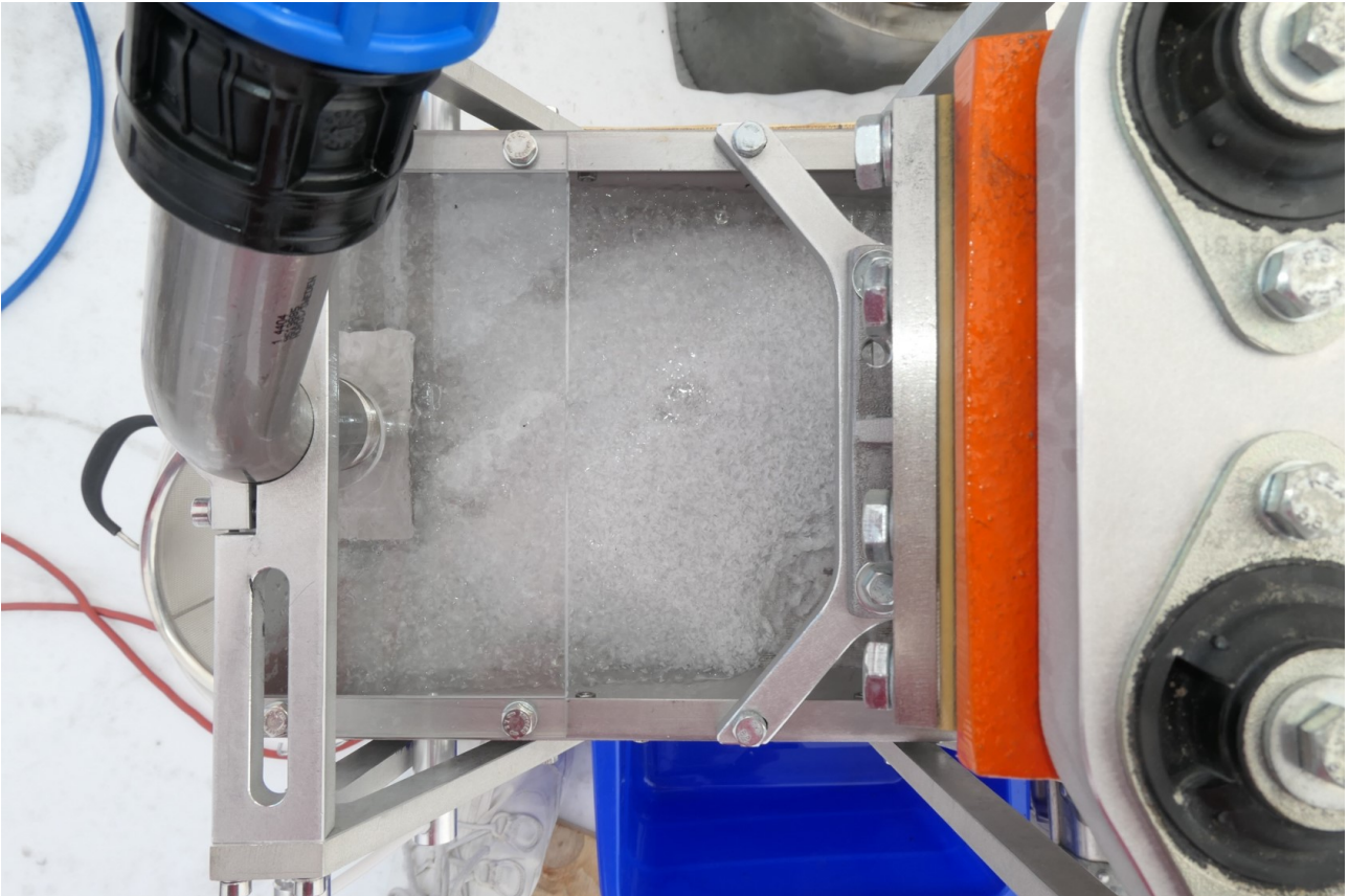
Ice chips freshly drilled by RADIX from a depth of 260 m. Photo: T. Stocker.
