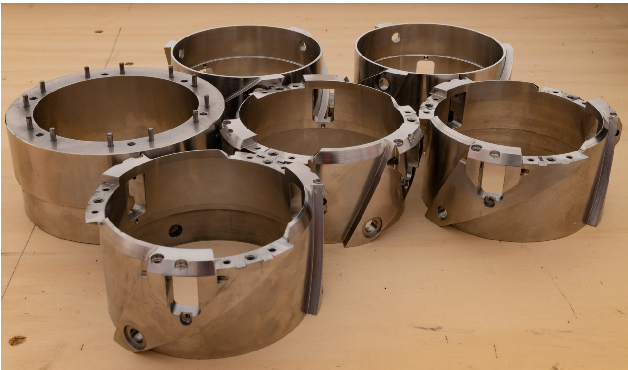
Collection of BEOIC drill heads made at AWI ready to be installed. Photo: C. Barbante (Leica SL2, 46 mm, f 22, 1/15 s, ISO-100).
