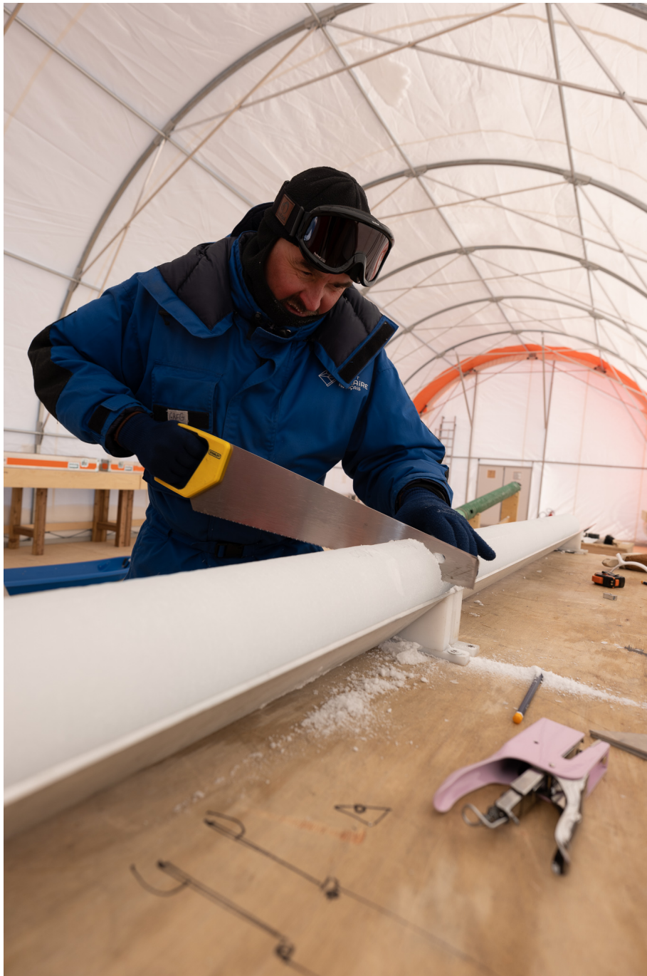
Greg Teste cutting the freshly drilled fir core from 102 m depth into 1-m pieces. Photo: T. Stocker
